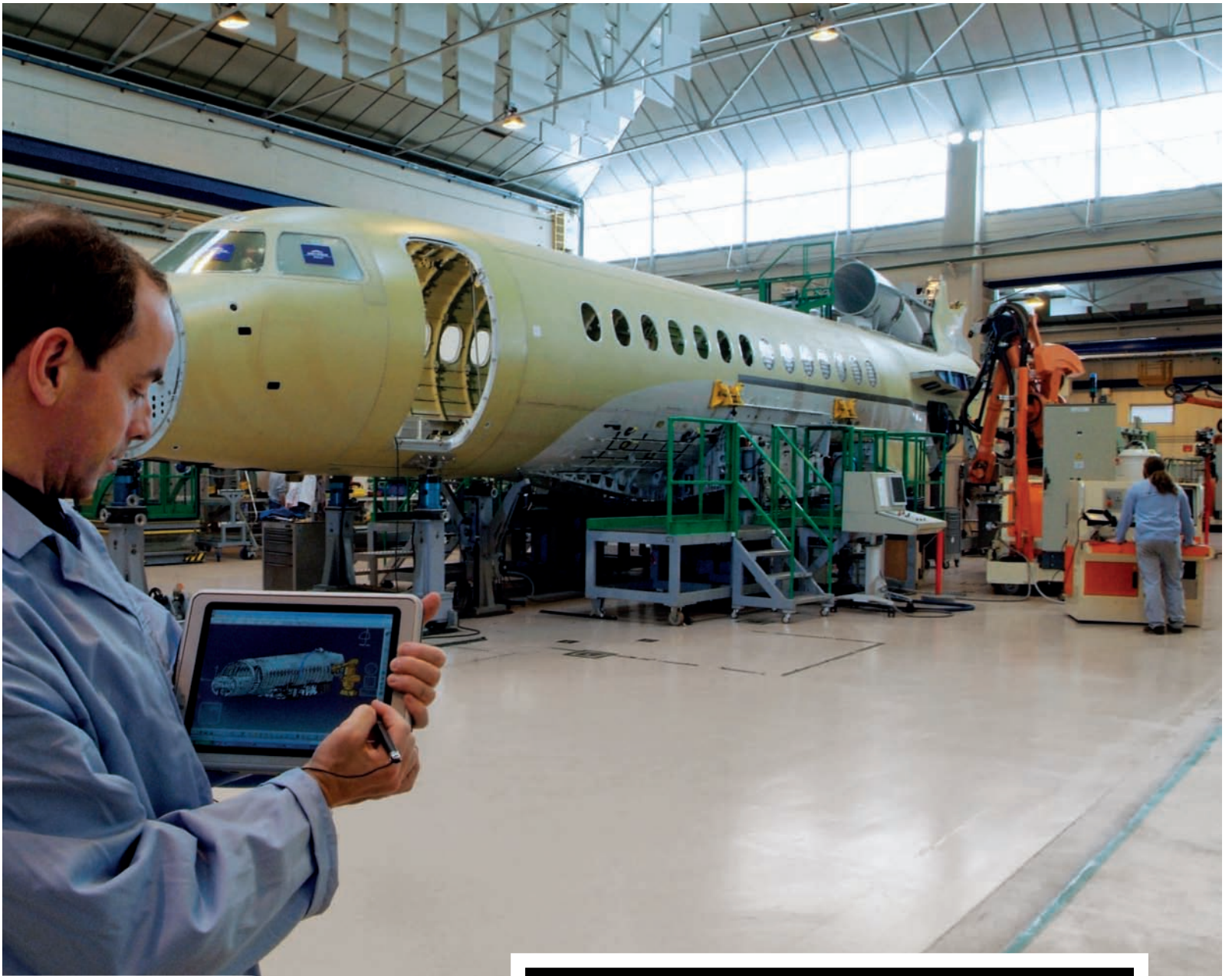
Biarritz: use of a tablet PC in the production of a Falcon 7X fuselage
