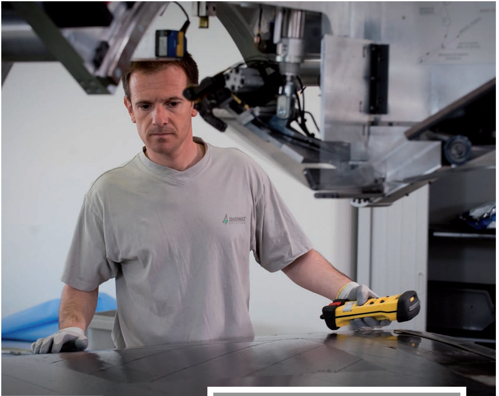
Biarritz: production of a Rafale wing out of carbon fiber
