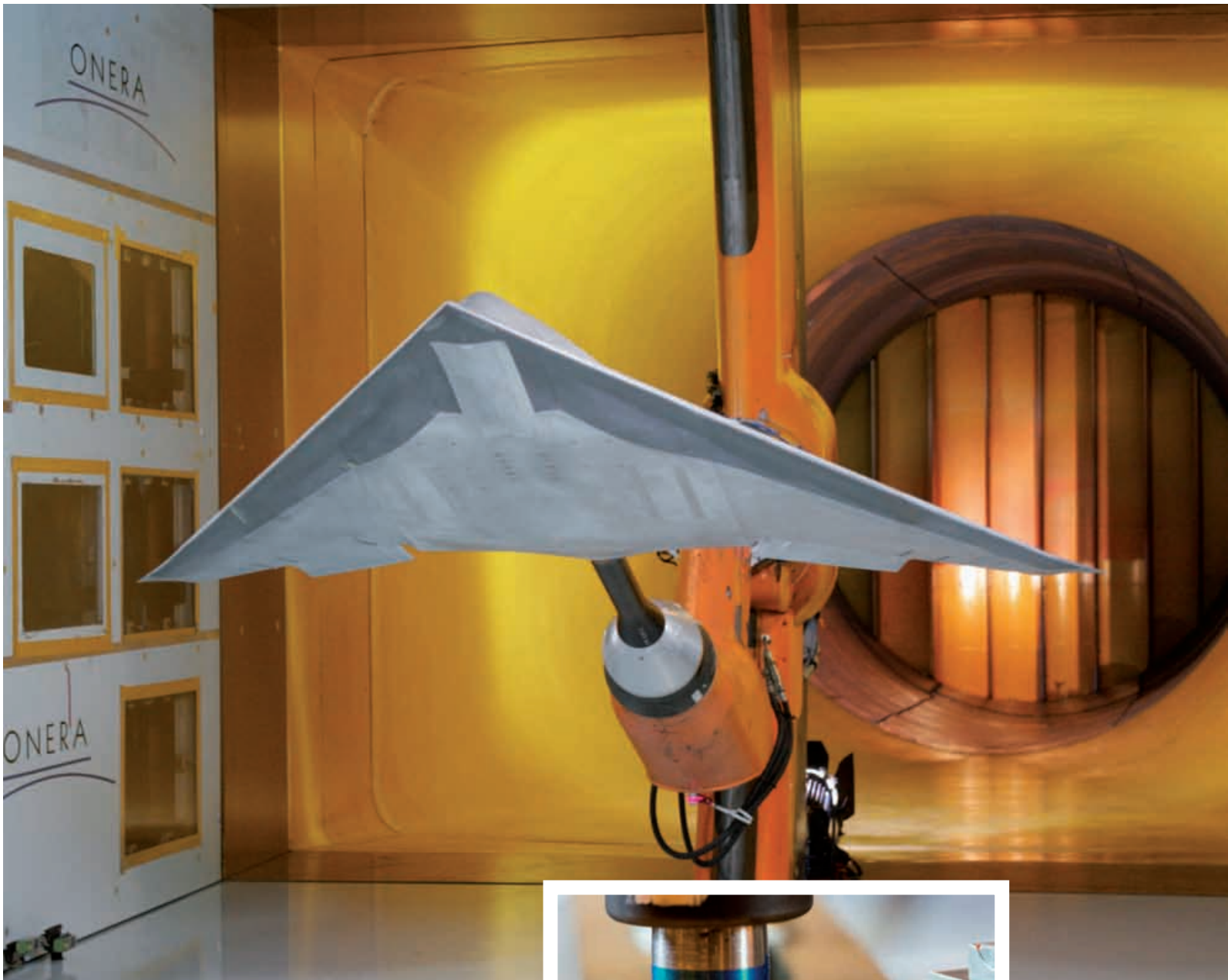
Research partnership with ONERA Wind-chamber testing of the nEUROn mock-up at ONERA.
