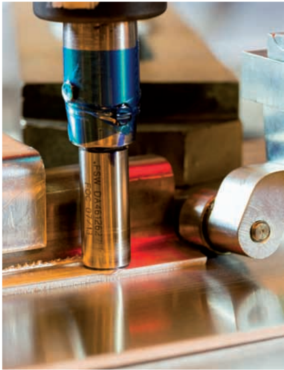
Friction-stir welding This green and silent technology enables the delicate welding – hitherto unrealizable – of high-resistance aluminum alloys.
