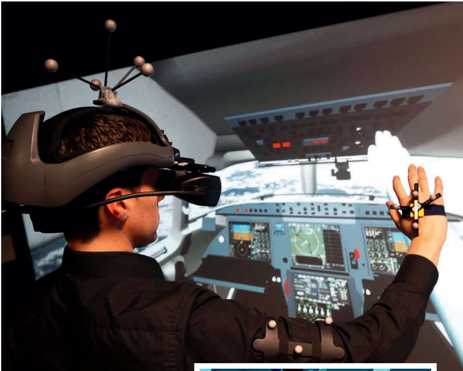
Immersive reality center at Saint-Cloud (Paris region) Thanks to this new tool, it is now possible to immerse oneself, in three dimensions and at full-scale, in the actual digital mockup and explore more rapidly a full set of solution combinations.
